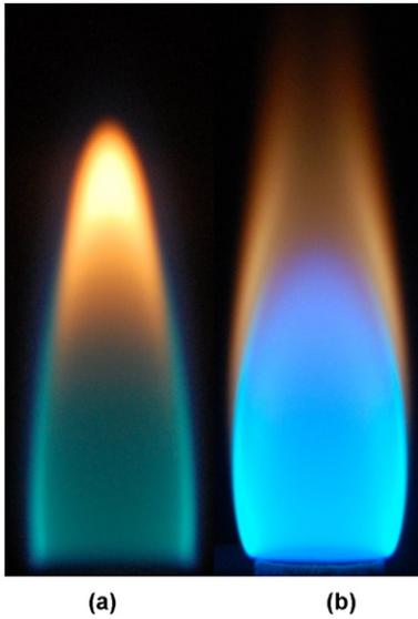
Fig. 2. Photographs of (a) normal and (b) inverse sooting limit flames. The sooting limit is observed at a height of 8 mm from the burner lip.
