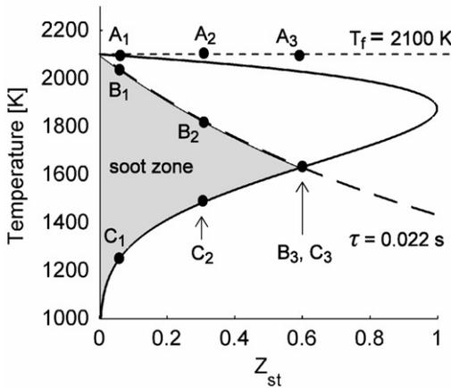
Fig. 6. Representation of the collapse of the soot formation zone with increasing  $Z_{st}$ .
