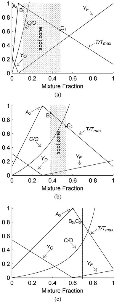
Fig. 7. Flame sheet model results for Cases 1, 2, and 3 from Fig. 6 showing shrinking of soot formation zone due to convergence of low-temperature ( $T_{kin}$ ) and low C/O ratio (high-temperature  $T_{C/O}$ ) boundaries.
