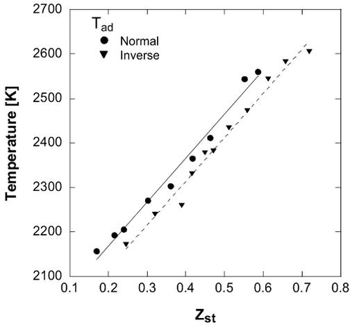
Fig. 4. Sooting limit flame temperature vs stoichiometric mixture fraction for normal and inverse flames. Case 2: Constant gas exit velocity.
