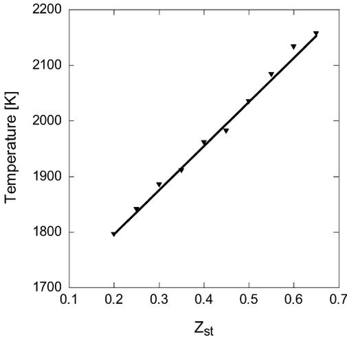
Fig. 5. Comparison of measured inverse flame sooting limits and the model (line) obtained with  $E_a = 31$  kcal/mol;  $C_0 = 780 \text{ K}^{-1} \text{ s}^{-1}$ ,  $\tau = 22.4$  ms and  $(C/O)_{cr} = 0.53$ .
