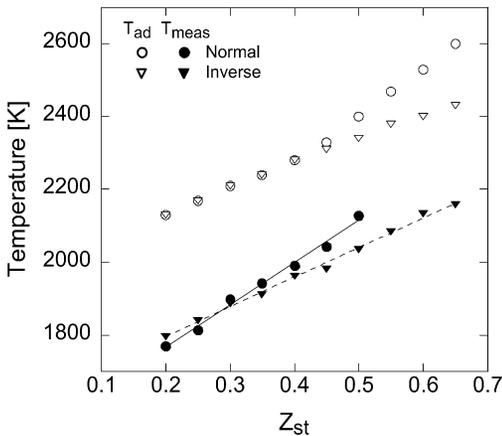
Fig. 3. Sooting limit flame temperature vs stoichiometric mixture fraction for normal and inverse flames. Case 1: Constant flame height of 16 mm.
