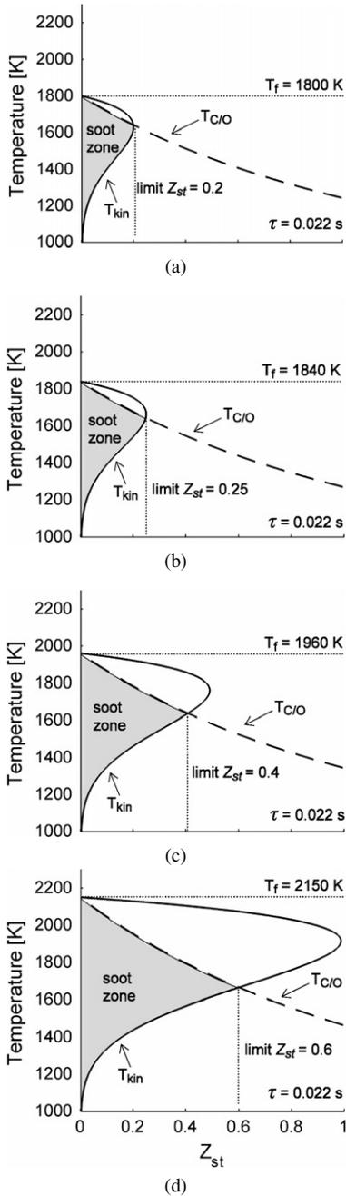
Fig. 8. Representation of the sooting zones of four flames with varying flame temperatures.
