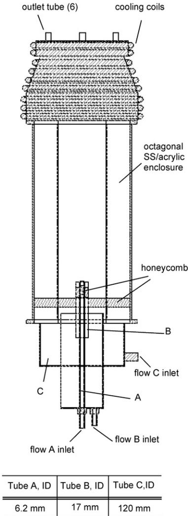
Fig. 1. Schematic diagram of burner for normal and inverse coflow flames.
